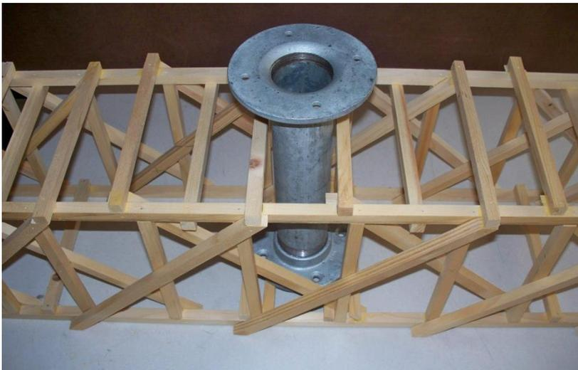
**Support flange placed inside of bridge shown above.
